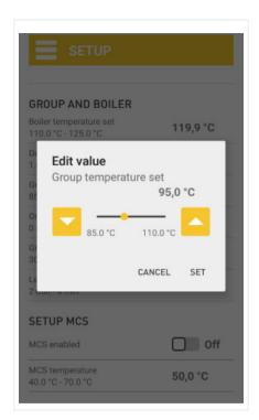
Off Energy saving 15:50 Time Date 07/06/15 **GROUP AND BOILER** Boiler temperature set 119,9°C 110.0 °C - 125.0 °C Delta T 2.0 °C 1.0 °C - 4.0 °C Group temperature set 95,0°C 85.0 °C - 110.0 °C On coffee 0 sec 0 sec - 30 sec Group delivery timeout 60 sec 30 sec - 120 sec Level timeout 3 mir 2 min - 4 min
